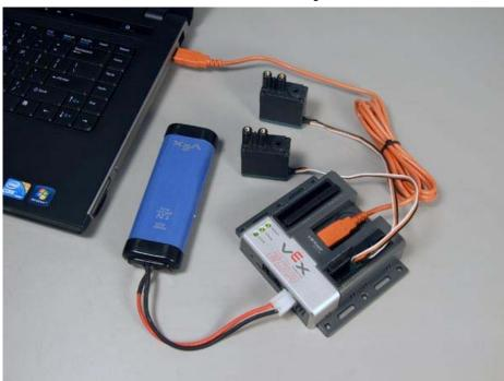
Note: Technically, the battery is not necessary for downloading Master CPU Firmware and ROBOTC Firmware, but it has helped in cases where the USB ports on the computer provide too little power to facilitate a reliable connection to the Cortex.
