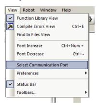
The Select Communications Port for Platforms window will appear. From the Communications Port drop down list, you should see "Automatic Selection" and one of two additional options:
