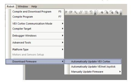
A message will appear, informing you that the software will update your Cortex to the latest Master CPU and ROBOTC Firmware files. Press OK to begin the process.
