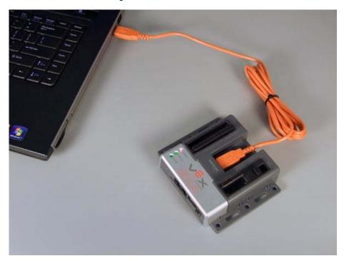
Connect a 7.2V Robot battery to the Cortex and move the POWER switch to the ON position. Optionally, you can connect two motors to MOTOR Ports 2 and 3 for testing a sample program later in the sequence. You can connect 3-wire motors directly, or the newer 2-wire motors using Motor Controller 29 cables.
