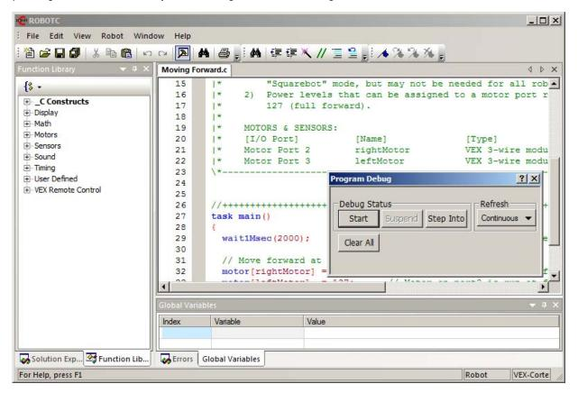
With the sample program above, you should observe motors plugged into Ports 2 and 3 spinning for 3 seconds.
