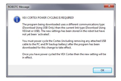
Once the program has downloaded to the Cortex, turn the Cortex off and back on. This 'power cycle' commits the communication type to the Cortex. Remember, you must repeat this process to revert back to USB only (making sure that USB only is selected as the mode). The Cortex should now be set up for wireless communication over VEXNet.
